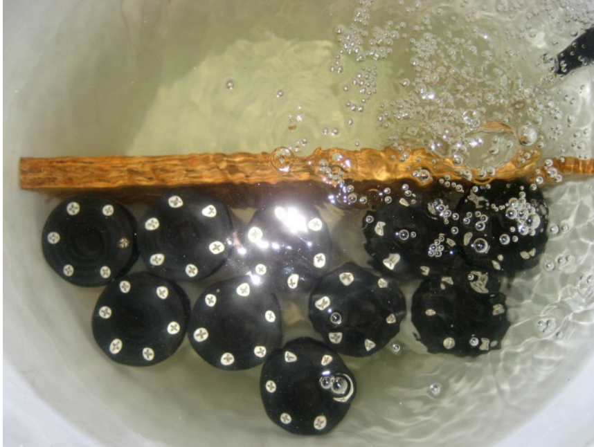
Figure 3. miniDOT verification procedure.
