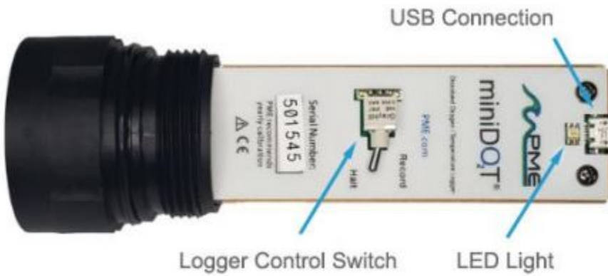
Figure 2. Internal miniDOT connections and controls.
